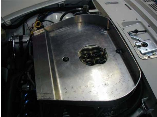
for the base leading edge. A simple wedge of aluminum will suffice and provide an extra measure of stability. Now drill 2 - 5/16<sup>th</sup> holes for drain tubes, one in the front and one in the rear, as well as the 5/8<sup>th</sup> inch hole for the breather tube hose on the drivers valve cover.
