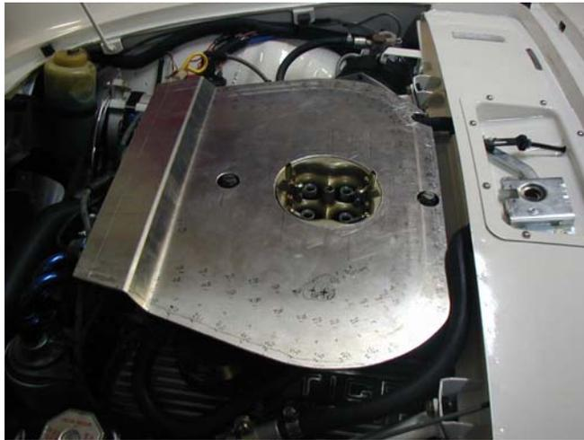
template to allow for the distributor cap to clear the base plate with a margin of safety. *(On the template I have available for others I traced the actual base bend side profile for reference.)*
