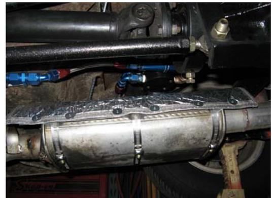
actually place my hand on the top surface of the muffler shield and it is hot to touch but NOT nearly the scalding hot it was before the shield was installed. That is around a 42% drop in the radiated heat and has sufficiently corrected the problem for me such that I am satisfied it will prolong the durability of my current fuel pump.
