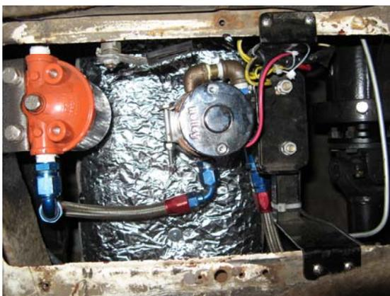
After installing the Reflecta Shield I then installed the shield assembly to the top of the muffler with the three included band clamps. In the photos you can see the Dan Walters Torque Arm assembly. The heat shield assembly has proven extremely effective and it has reduced the muffler radiated temperature by roughly 87 degrees from muffler temp radiating from the top of 210 degrees to radiant heat of roughly 123 degrees. I can
